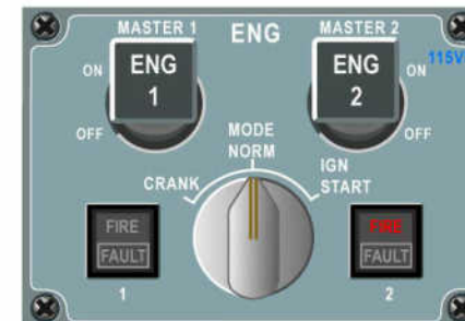
Figure 14 Operation of the Fire Extinguishing System (1)
