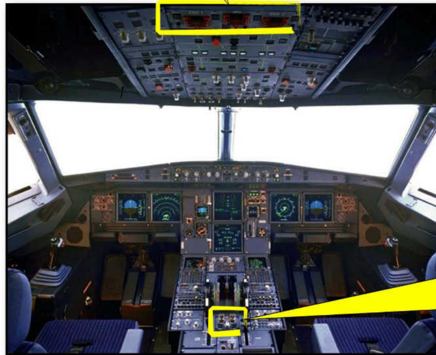
Figure 20 Engine Fire Component Location
