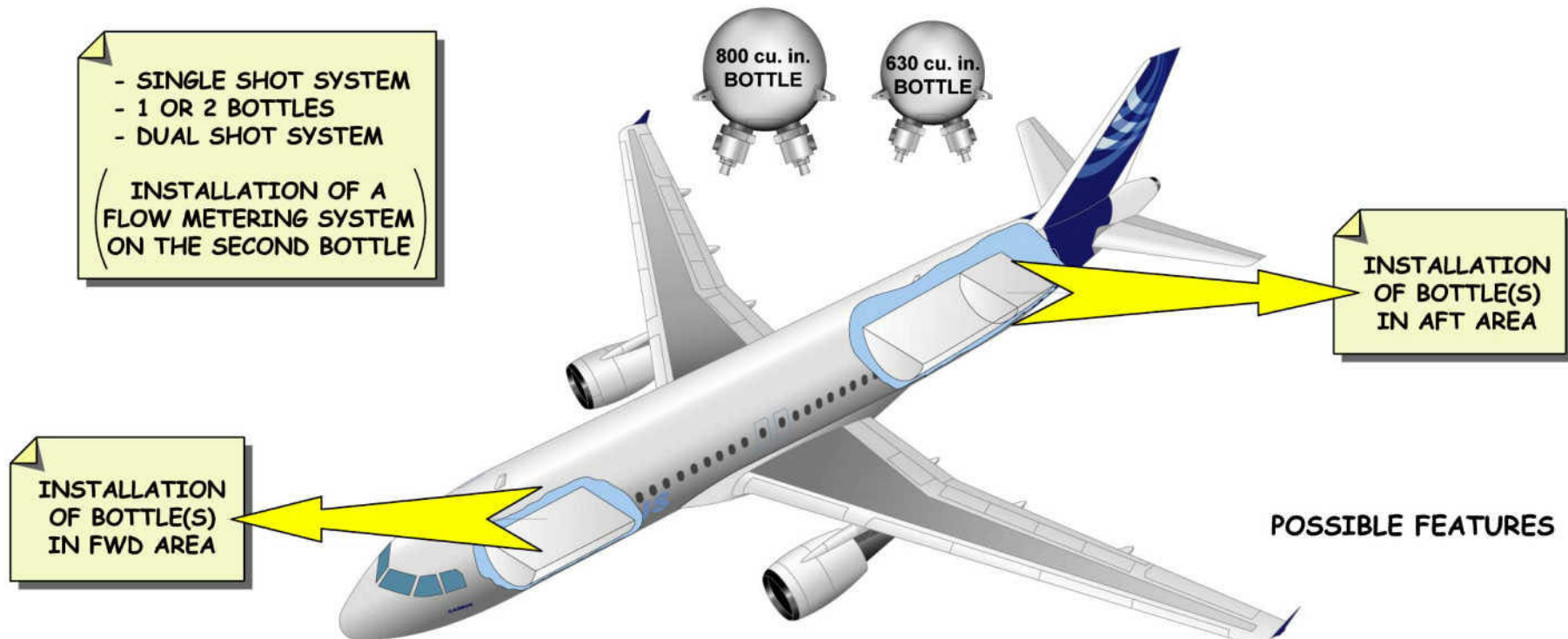
Figure 59 ETOPS Requirements for Cargo Hold Protection
